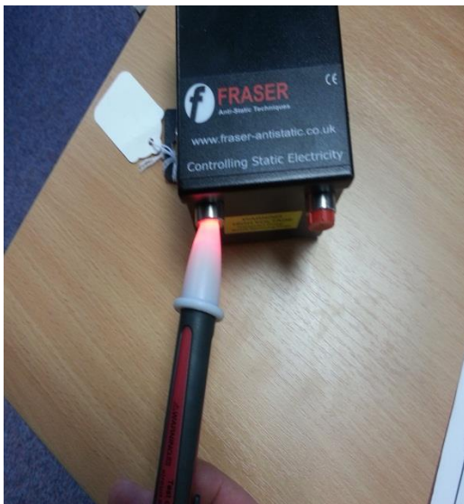
Figure 3. Volt Stick verifying that High Voltage Output is present, use a piece of earth cable if Volt stick is not of suitable length to access the power supply port (only touch the insulated part of the cable)
