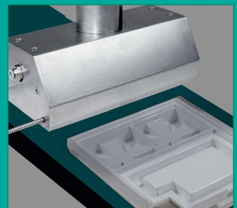
Cleaning (e.g. PCBs) with ionized air and rotating nozzles with a simultaneous vacuum aspiration
