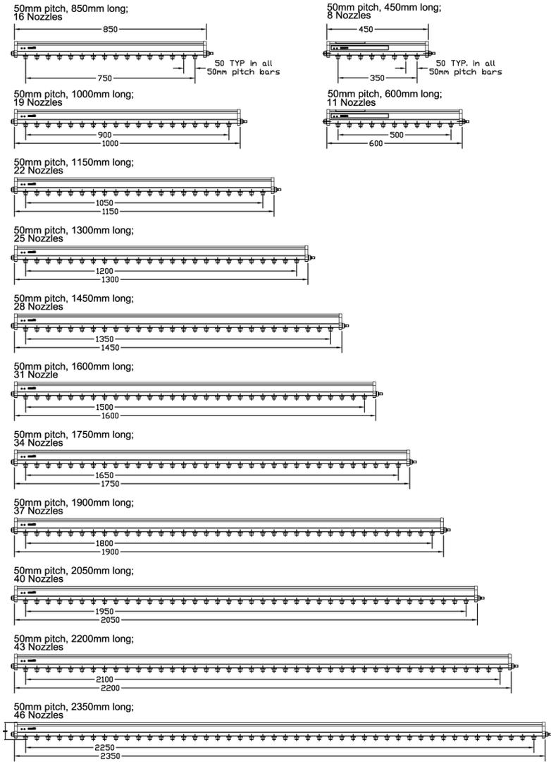
Figure 10. Model 5635 Lengths with 50 mm and 75 mm Emitter Pitch Spacing
