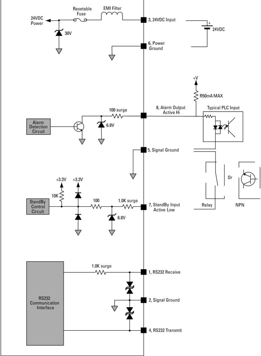
Figure 5. Model 5635 Wiring Diagram
