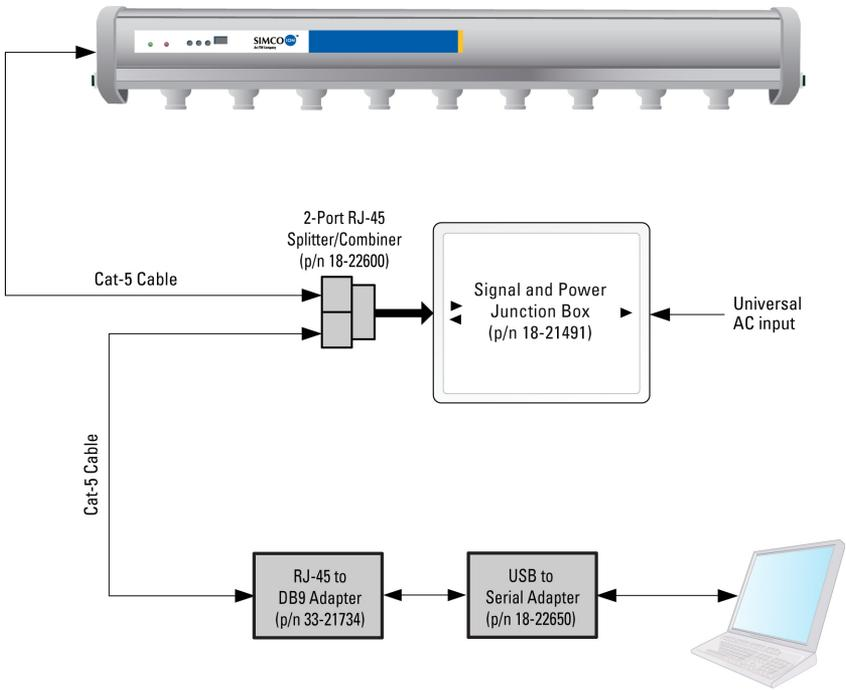
Figure 3. Hard Wire to Junction Box and +24 VDC Tool Power
