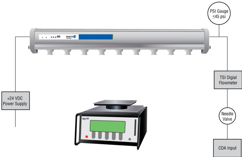
Figure 9. Recommended Setup for Calibration
