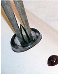
Figure 15. Removal of Silicon Emitter Point
