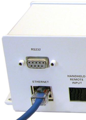
Figure 7. CAT-5 Cable Connected to Ethernet Port
